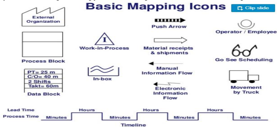
Fig 6: Basic symbols in value stream mapping
